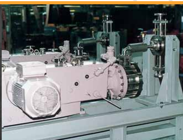
Pumping of oxazolidone at 200°C
